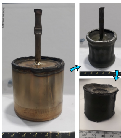
Figure 5 Photographs of: Packed canister (left), HIPed canister (top right) and Cs-chabazite HIPed wasteform (bottom right)
